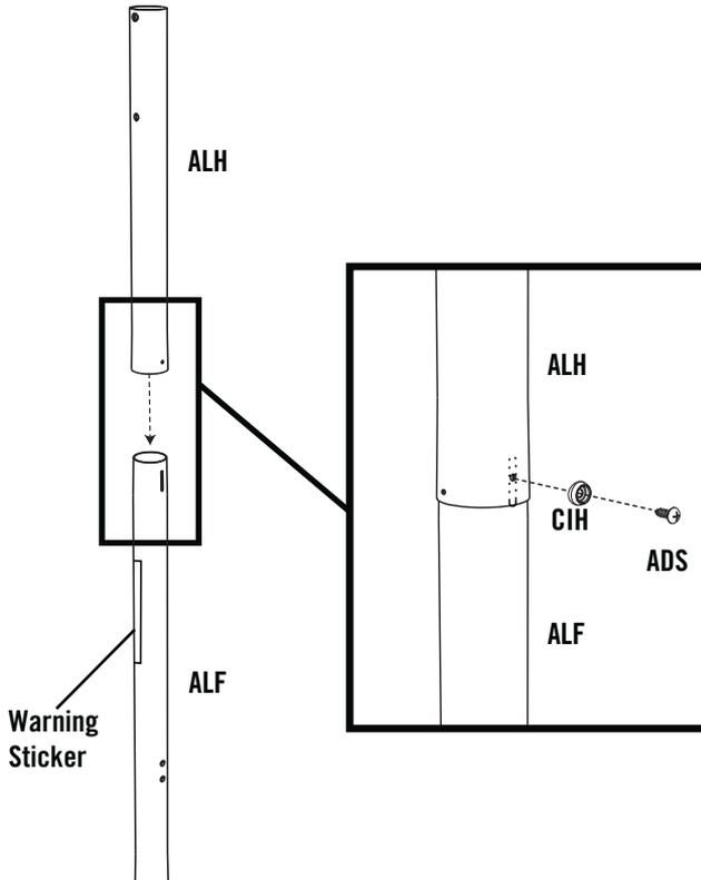
**!** *Note: The 1/4" x 3/4" Screw and Domed Countersink Washer should be flush with the Pole, but will spin freely once installed. Do not jam the Poles together until instructed.*
